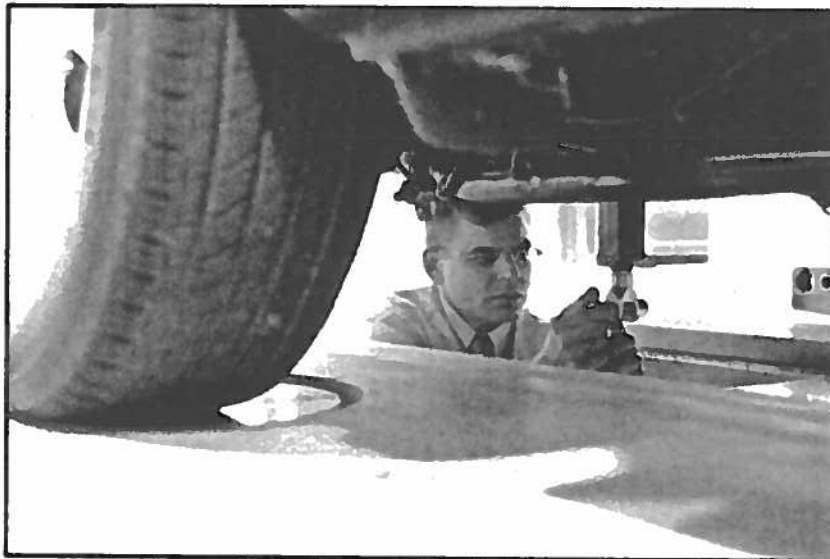
The CU-ICAR CoEEs feature state-of-the-art research equipment. BMW Automotive Manufacturing Chair Tom Kurfess is shown here using the Zeiss Pro T Compact Dual Column Full Vehicle CMM, a drive-on research tool to allow full vehicle and other large-item coordinate measurements.
