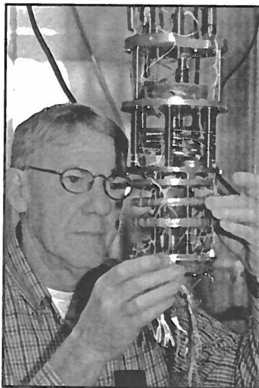
Dr. Richard Webb, CoEE Endowed Chair in Nanoelectronics, works the sample wiring for his ultra-low temperature dilution refrigerator, which is capable of cooling samples to 0.003 Kelvin. This machine is equipped with two superconducting quantum interference devices (SQUIDs) used for thermometry as well as an 8 Tesla superconducting magnet.
