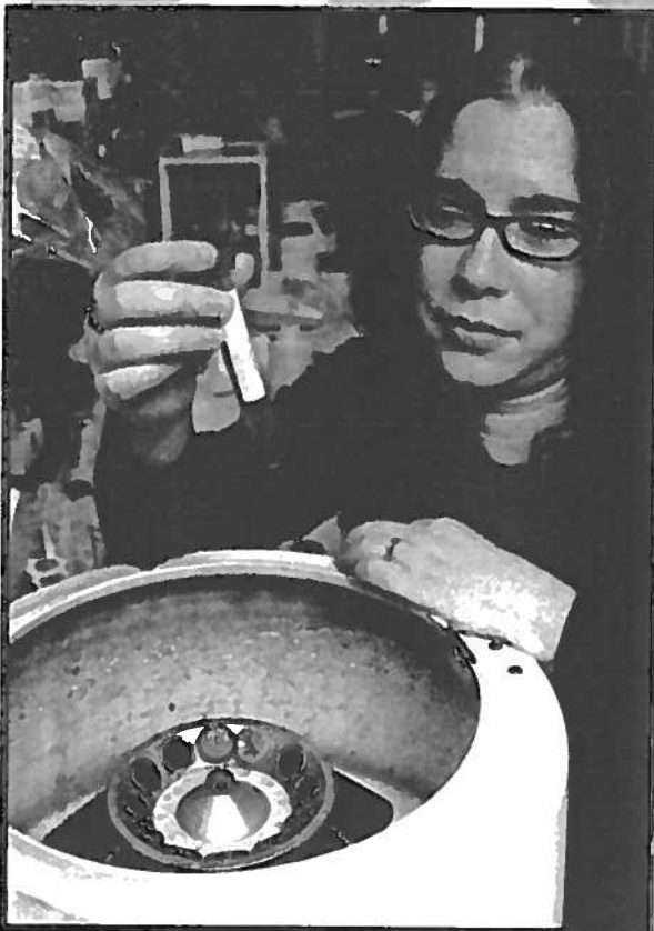
Dr. Cathy Murphy of the Nanoenvironmental CoEE removes solutions of purified gold nanorods from a centrifuge. These nanorods can be used as therapeutics to eliminate bacteria in the human body with the use of lasers.
